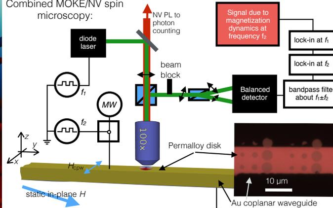
1. Differential MOKE microscopy measures difference in  $\vec{M}$  between two values of  $H_{cpw}$ . [1]
